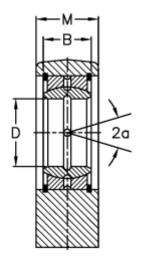
= 110 Α a (degrees) = 7 В = 32 D = 45 Dynamic load C (kN) = 127F = 77 L = 132
